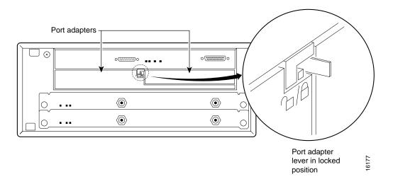
**Note** If the port adapter lever does not move to the locked position, the port adapter is not completely seated in the midplane. Carefully pull the port adapter halfway out of the slot, reinsert it, and move the port adapter lever to the locked position.
